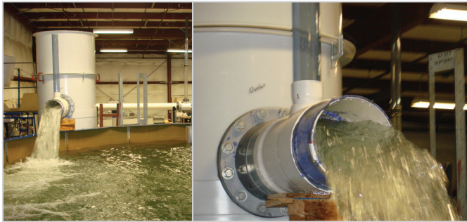
Fig.4 Grab samples were collected from the influent (not pictured) and effluent (above) over a range of hydraulic loading rates.
